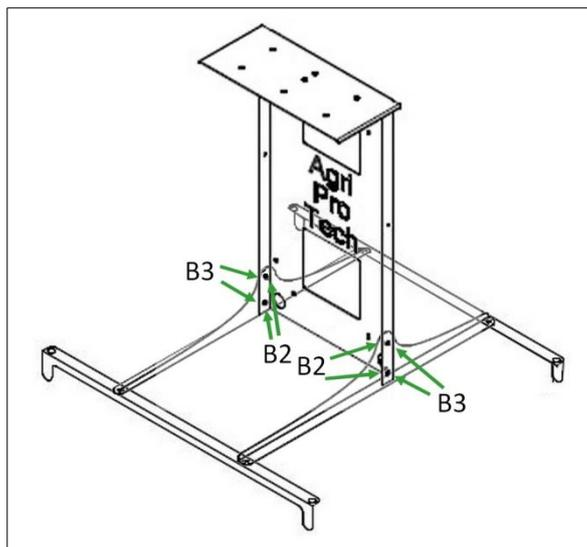
Picture 4 Screw the rear plate to the feet and rails
