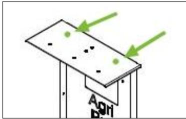
Picture 8. Holes for speaker on AviTrac® 18M
