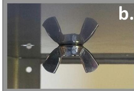
Picture 7. Wing nut position and speaker screw
