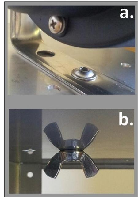
Picture 10. Wing nut position and speaker screw
